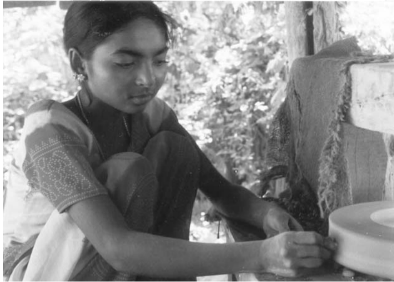
Figure 1. Agate worker shapes a stone on a horizontal grinding wheel.
